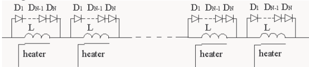
Figure 5: Magnet string with the cold diodes.
