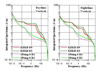
Figure 4: Integrated spectra for vertical GM in the daytime and night-time at KEKB and SPring-8 (Vertical)
