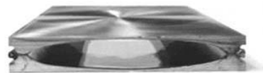
Fig.10. A test model of ID duct. The inner surface is coated with Cu.
