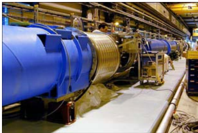
Figure 5: Prototype jacks under String-2 at CERN.
