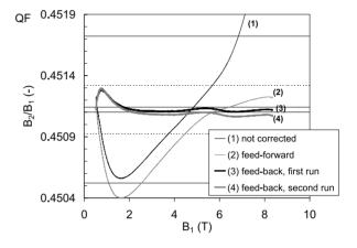
Figure 2: Ratio  $B_2/B_1$  for the QF quadrupole, plotted as a function of the dipole field along the reference current ramp.
