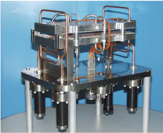
Figure 4: Completed MEBT-chopper structure assembly.
