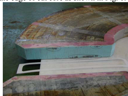
Fig. 6. Cut core gap after 8 hours power test. The places touched by water directly are cooled (light blue colour).
