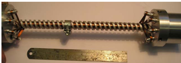
Figure 9: Prototype model of a superconducting undulator for a polarized positron source (Daresbury).
