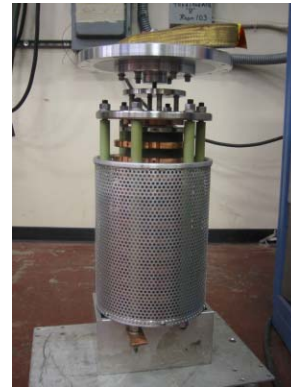
Figure 9: A coaxial modified structure matching resistor picture.
