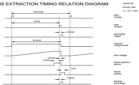
Figure 1: SNS Accumulate Ring Extraction Kicker System pulses timing relation
