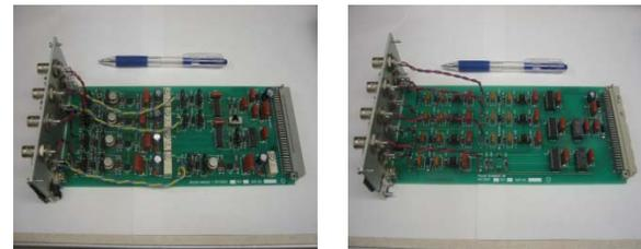
Figure 6: fan out board and summing board pictures
