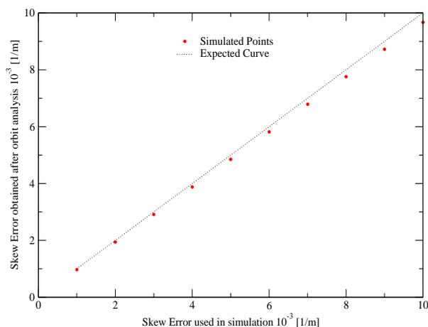
Figure 3: Relation between the skew quadrupole errors used to generate the RHIC orbits and the skew quadrupole errors recovered using the action and phase analysis on the simulated orbits.
