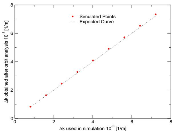
Figure 2: Relation between the gradient errors used to generate the RHIC orbits and the gradients errors recovered using the action and phase analysis on the simulated orbits.
