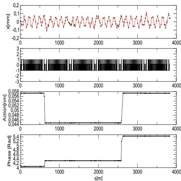
Figure 1: Action and phase analysis on a RHIC simulated orbit. One gradient error as big as  $10^{-3}$  1/m has been introduced intentionally in the simulation
