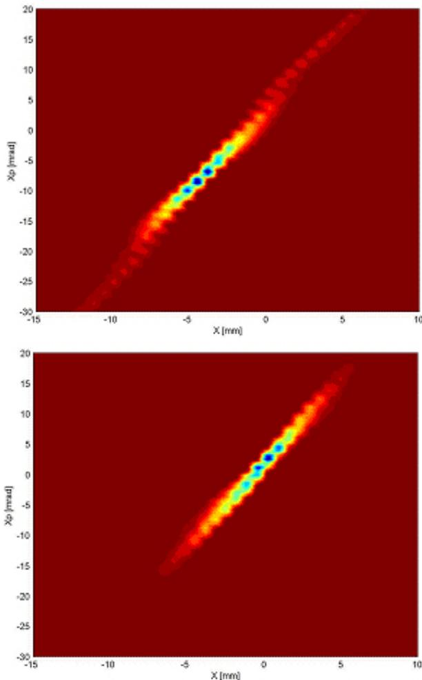
Figure 3: Horizontal emittance plots of the nominal MEBT optics (the top plot) and the round beam optics (the bottom plot). The halo is visibly reduced. The rms emittance is reduced from 0.593 mm-mrad to 0.376 mm-mrad.
