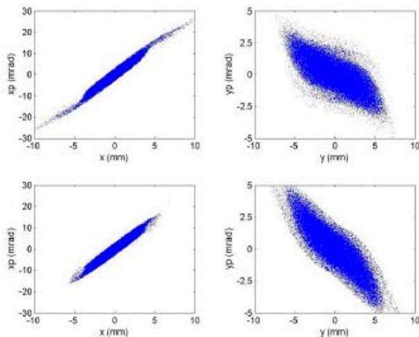
Figure 5: Plots of simulated beam distributions. Upper plots are obtained using the nominal MEBT optics and lower plots using the round beam MEBT optics. Reduction in halo is visible in both planes.
