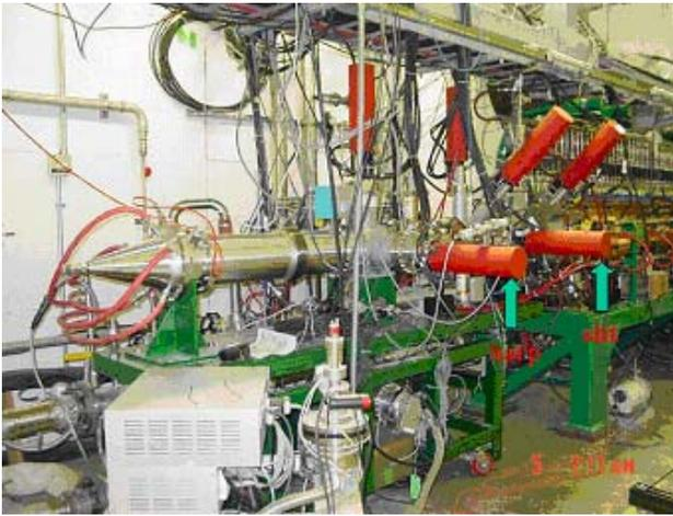
Figure 2: Photo of the Diagnostics plate attached at the end of DTL tank 1. The beam direction is right to left.
