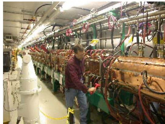
Figure 8: CCL magnet alignment.
