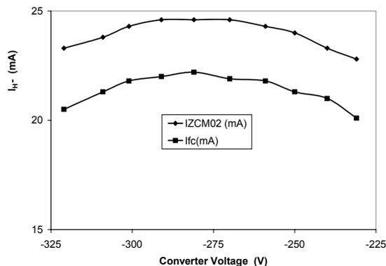
Fig. 3. Plot of the experimentally measured  $\text{H}^-$  currents from the development source.
