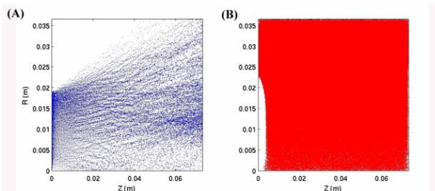
Fig. 5. Preliminary 2-D PIC code simulation for  $H^-$  beam being accelerated off the surface converter located on the left in Figs. 5(A) and (B). Fig. 5(B) shows the plasma electrons, and formation of the sheath at about 3 mm from the converter.
