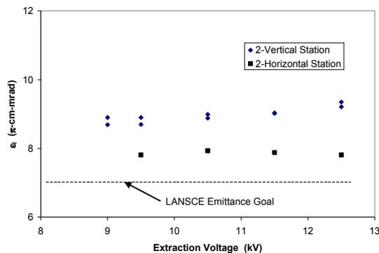
Fig. 4. Plot of 95% beam fraction laboratory emittance for 20 mA  $\text{H}^-$  beam from the development source.
