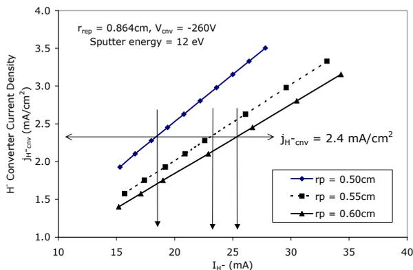
Figure 2. PBGUNS predictions for 80keV  $\text{H}^-$  current and  $j_{\text{H}^- \text{cnv}}$  at a  $\text{H}^-$  sputter energy of 12eV.
