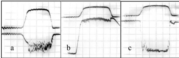
Figure 4: Oscillograms: a – the field in the fifth resonator (upper ray) and the field in the first resonator (lower ray) at the moment of instability appearing; b – the field in the fifth resonator and the injector current at BCT (38 mA/div , 0.5  $\mu$ s/div); c – the field in the fifth resonator and the current on the Faraday cup (37 mA/div , 0.5  $\mu$ s/div).
