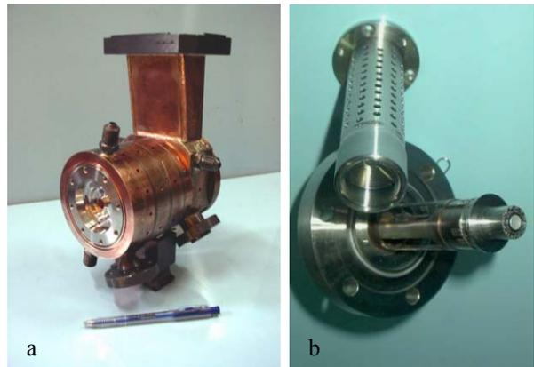
Figure 1: a – The bunching system; b – the cathode assembly and the focusing electrode.
