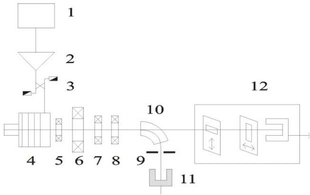
Figure 3: The testing stand scheme: 1 klystron modulator; 2 klystron ( $P_{out}=16$  MW,  $\tau=2,2$   $\mu$ s); 3 directional coupler (-10 - -22 dB); 4 injector; 5 beam current transformer (BCT); 6 axially-symmetric lens; 7 quadruple lens; 8 the beam position adjusters; 9 collimator; 10 magnetic analyzer; 11 Faraday cup; 12 the beam transverse distribution and emittance measurement system.
