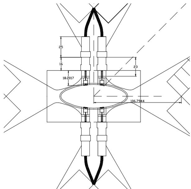
Figure 4. Layout of pick-up monitor installation in NESTOR.
