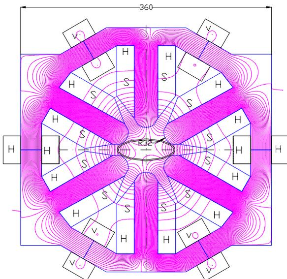
Figure 3. Layout of sextupole magnet with corrector coils.
