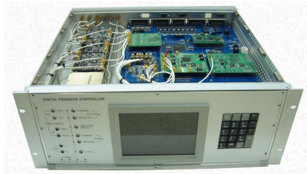
Figure 4: Photograph of the digital RF feedback controller for PEFP 100MeV Proton LINAC.
