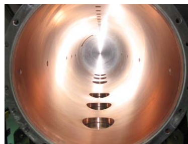
Figure 1. Plated inside of tank.
