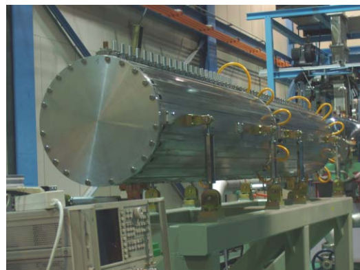
Figure 2. Installed DTL tank 1.
