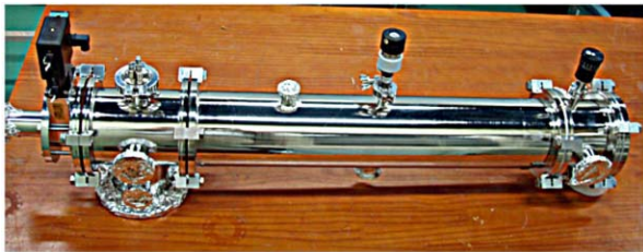
Figure 5. Energy monitor to measure the beam energy of the RFQ.
