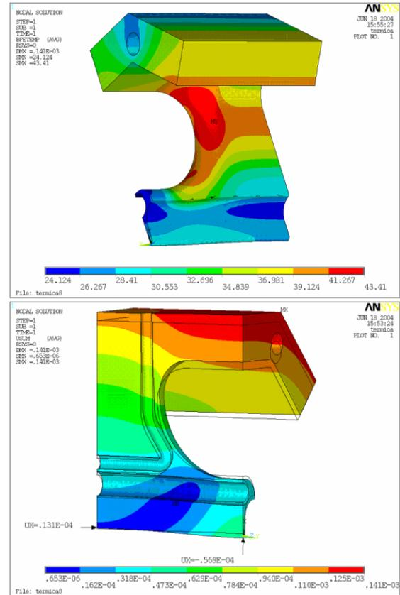
Figure 7: Temperature in °C and deformations in meters.
