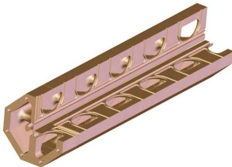
Figure 3. Geometry of one RFQ module (1.5 m long).
