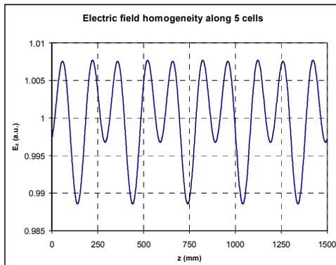
Figure 6: longitudinal  $V(z)$  variation along 5 cells.
