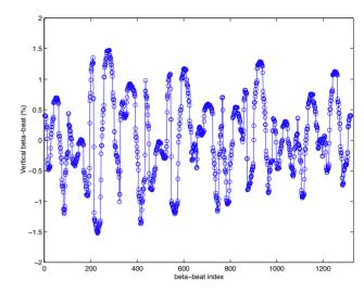
Figure 7: Vertical beta beating in (%) for the June 2004 model optics.
