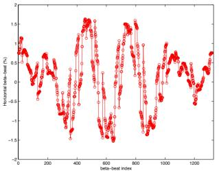
Figure 6: Horizontal beta beating in (%) for the June 2004 model optics.
