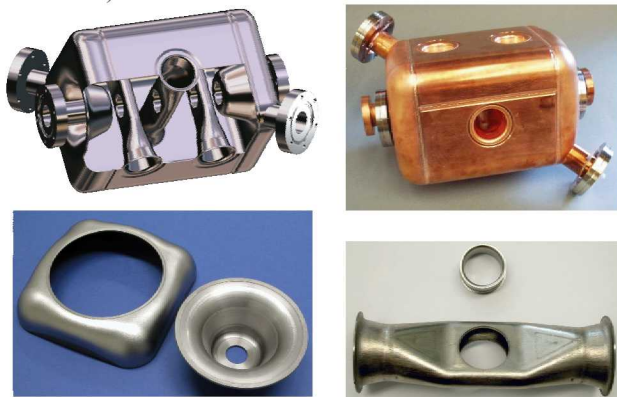
Figure 1: Triple-spoke cavity prototype – artistic view, copper model and Nb parts.
