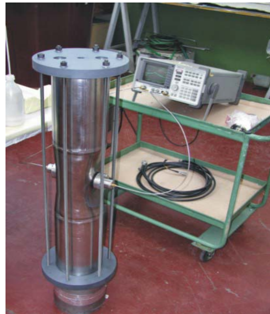
Figure 2: Frequency check of the unwelded parts at ZANON
