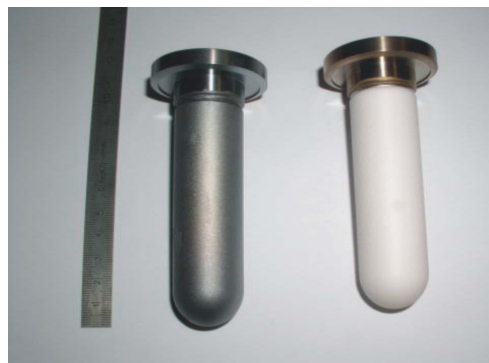
Figure 5: Cold window before (right) and after Ge plating (left)
