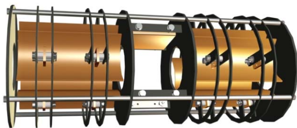
Figure 4: Electrostatic quadrupole doublet with integrated steerer
