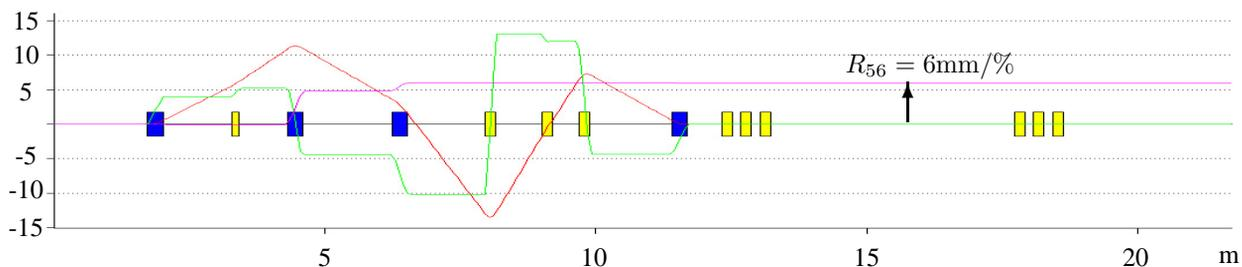
Figure 4: XBEAM Simulation: Dispersion  $R_{16}$  (red) in mm/%,  $R_{26}$  (green) in mrad/% and  $R_{56}$  (purple) in mm/%
