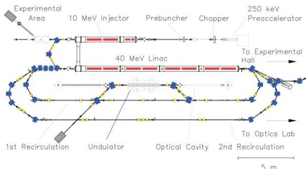
Figure 1: Accelerator Hall of the S-DALINAC
