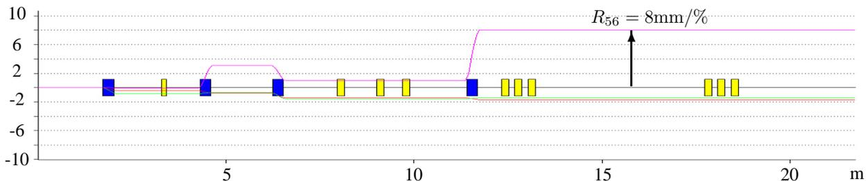
Figure 5: XBEAM Simulation: Dispersion  $R_{16}$  (red) in mm/%,  $R_{26}$  (green) in mrad/% and  $R_{56}$  (purple) in mm/%
