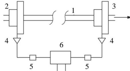
Figure 3: Set Up of the Energy Measurement: 1. Beam Tube, 2. Reference Monitor, 3. Measurement Monitor, 4. Amplifier, 5. Microstrip Filter, 6. Gain/Phase Detector.
