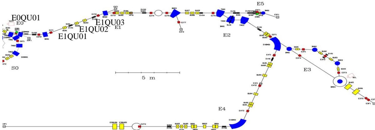
Figure 2: Extraction of the S-DALINAC: E0 Ejection, E1 Beam Optics, E2 40°-System, E3 QCLAM Spectrometer, E4 Energy-Loss Spectrometer, E5 High Energy Experimental Site.
