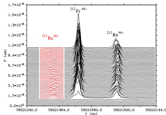
Figure 2: Waterfall diagram of the Schottky noise of a fragment beam with stochastic pre-cooling and subsequent electron cooling. The signal from  $^{212}\text{Ra}^{86+}$  could not be detected with electron cooling only.
