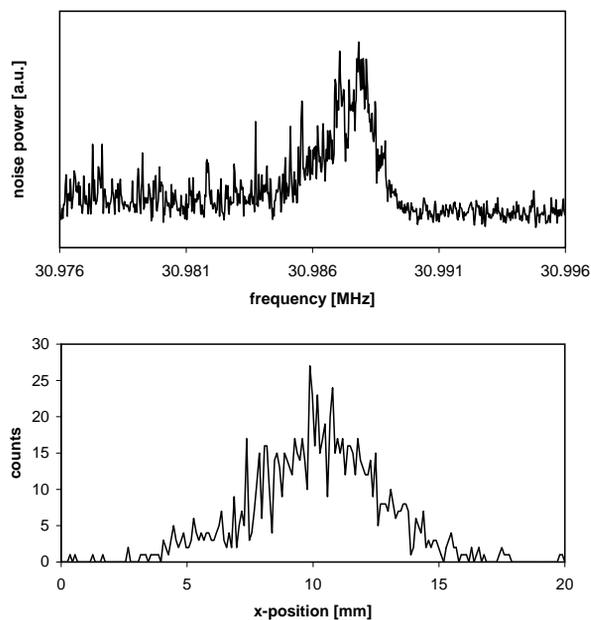
Figure 1: Measurement of a bare uranium beam at 3 MeV/u cooled with an electron current of 5 mA. The longitudinal Schottky spectrum measured at the  $140^{th}$  harmonic of the revolution frequency corresponds to a momentum spread of  $1 \times 10^{-4}$ . The residual gas ionization monitor measured a beam width of 5 mm.
