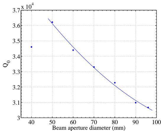
Figure 6: Drift-tube cavity -  $Q_0$  vs. beam aperture diameter.
