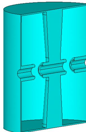
Figure 1: Cross section of the generic half-wave resonator.
