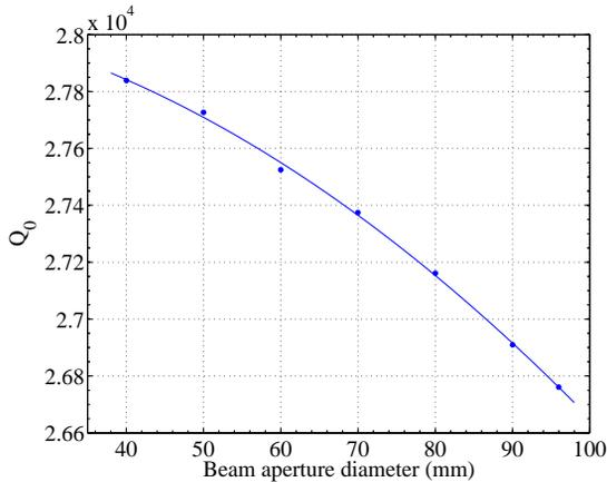
Figure 2: Half-wave resonator -  $Q_0$  vs. beam aperture diameter.
