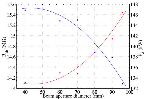
Figure 3: Half-wave resonator -  $R_{sh}$  and  $P_d$  vs. beam aperture diameter.
