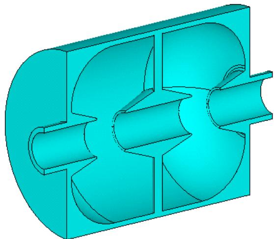
Figure 5: Cross section of the generic drift-tube cavity.
