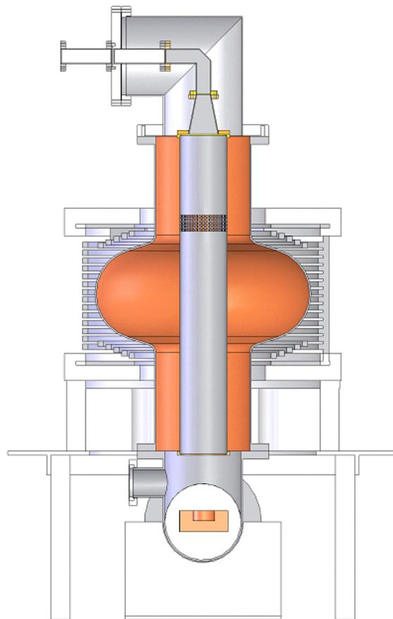
Figure 4: ECR plasma creation inside an elliptical cavity
