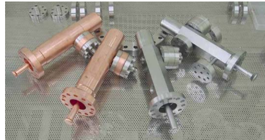
Figure 6: Four types of HOM couplers.
