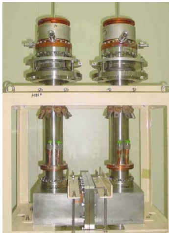
Figure 4: Input couplers at the test stand.
