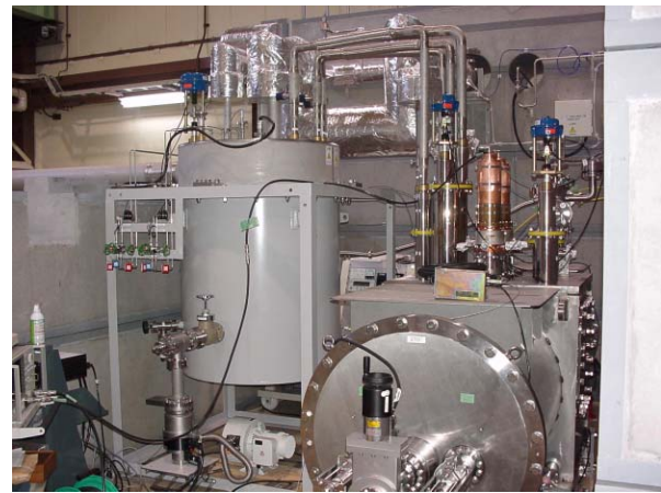
Figure 3: Valve box and cryomodule.
