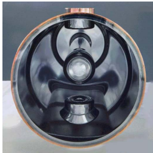
Figure 1: A medium \beta QWR after being Nb sputtered
