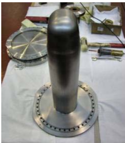
Figure 4: The tapered inner conductor before welding.
