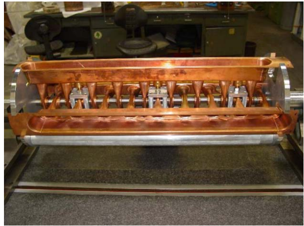
Figure 4: Due to the complicated fabrication process every step has been performed in copper first.
