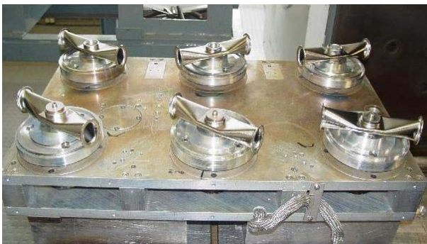
Figure 3: Preparation of stems and drift tubes for electron beam welding.
