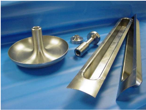
Figure 2: End-caps with drift tubes and girders made from bulk niobium.
