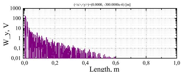
Figure 3: Transverse wake potential of VP-modes.
