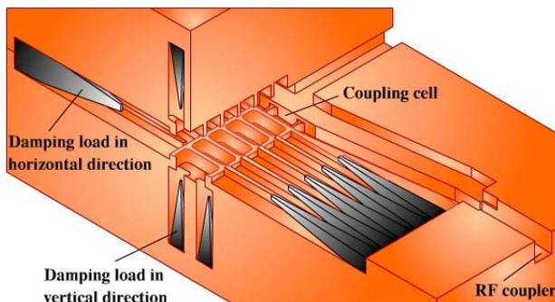
Figure 1: The planar 30 GHz accelerating structure.
