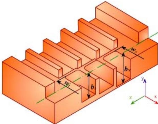
Figure 5: Detuned planar accelerating structure.
