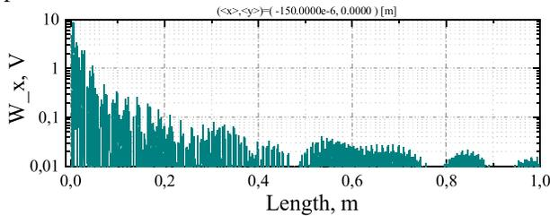
Figure 6: Transverse wake potential of HP-modes.
