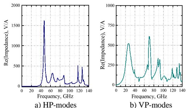
Figure 4: Real part of the longitudinal impedance.
