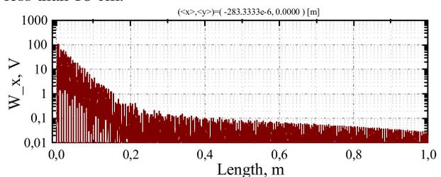
Figure 2: Transverse wake potential of HP-modes.
