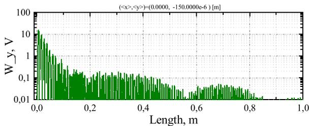
Figure 7: Transverse wake potential of VP-modes.
