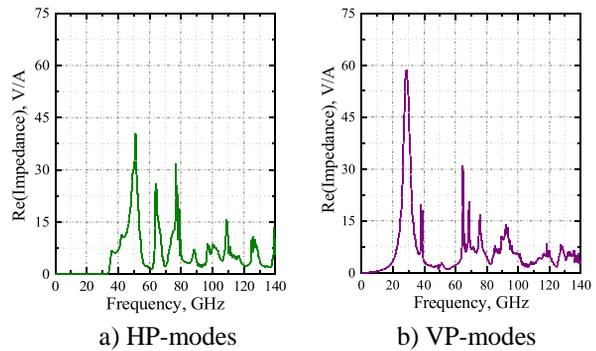
Figure 8: Real part of the longitudinal impedance.
