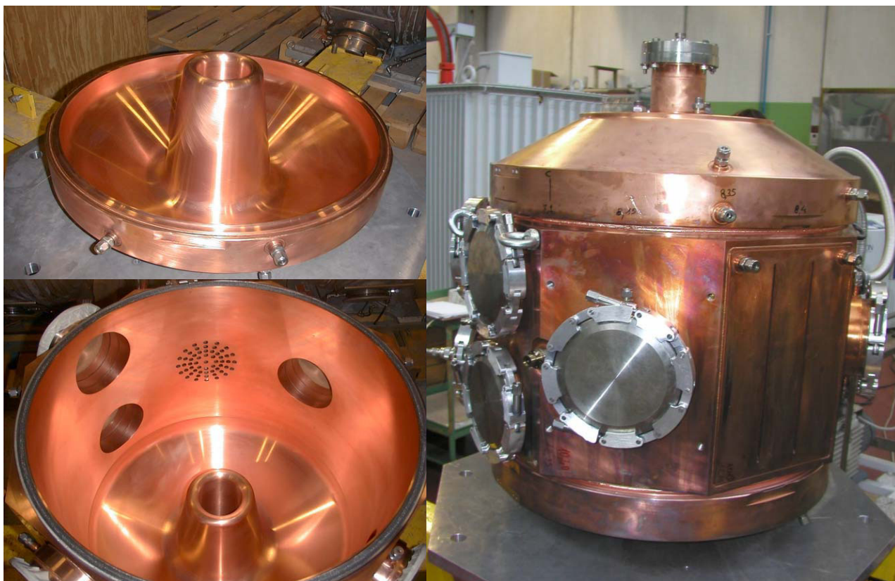
Fig. 2: a) The end-cap with the nose cone; b) the central part on the nose cone, c) the three pieces assembled vertically before machining and welding in order to perform the measurements.
