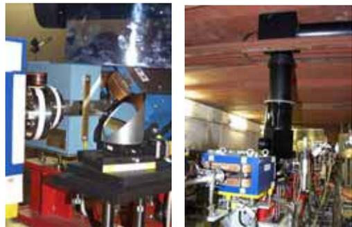
Figure 5: Two views of the beamline for FIR and optical radiation installed at the bunch compressor.
