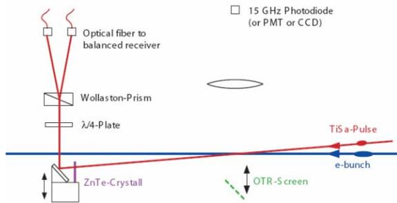
Figure 6: Principle of the EOS experiment.
