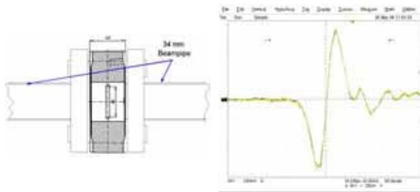
Figure 4: The TTF2 phase monitor (left), constructed as a thick, double-sided flange (40 mm) between two beam tubes. The signal of this monitor (right) was measured with a scope with 10 GHz analogue bandwidth.
