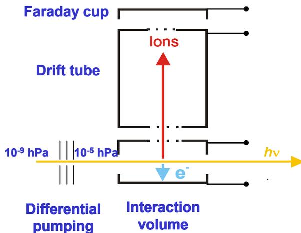
Figure 10: Gas ionisation detector to monitor the radiation pulse energy.
