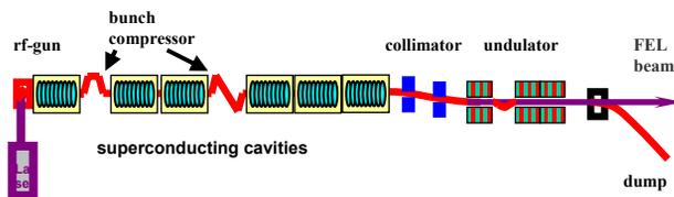
Figure 1: Schematic layout of TTF2.
