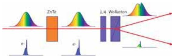
Figure 7: Principle of the time-to-frequency conversion.
