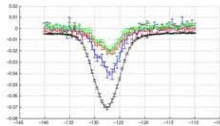
Figure 8: Variation of the FIR intensity with the RF phase of the acceleration structure measured with different detectors in the TTF2 bunch compressor.
