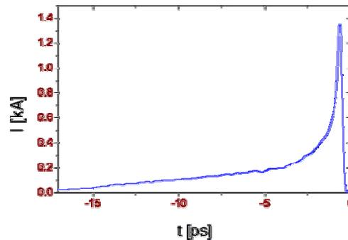
Figure 3: The electron distribution within a bunch simulated for TTF1. Lasing is supported only by the small fraction of the charge in the narrow spike produced by the bunch compressor [2].
