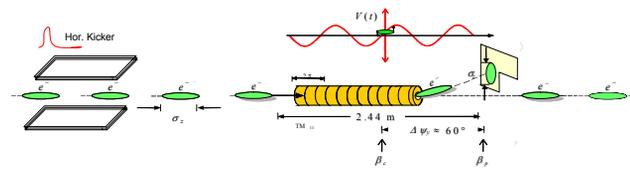
Figure 9: Scheme of electron bunch streaking by a transverse mode cavity.
