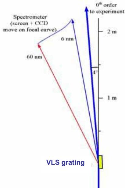
Figure 11: Scheme of the VLS grating spectrometer for the online measurement of single pulse radiation spectra.
