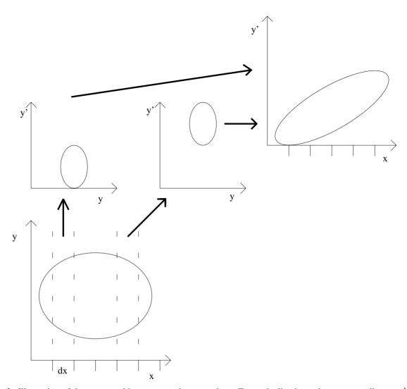
Figure 2: Illustration of the tomographic reconstruction procedure. For each slice in x, the corresponding y-y' phase space is reconstructed. Each of these is projected onto the y' axis, before they are combined into the x-y' phase space distribution.
