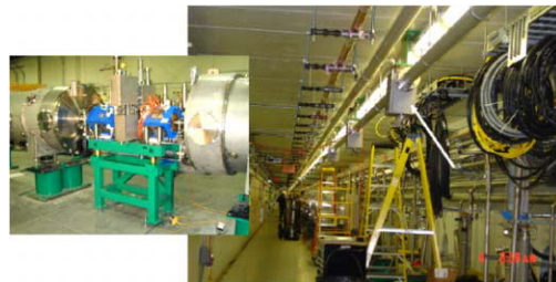
Figure 2. The optical transfer line in the tunnel and beam optics box setup (insert).
