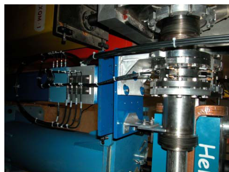
Figure 1. This XDKI BPM (oriented vertically in figure) is shown with its associated verification hardware.
