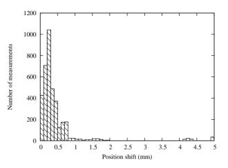
Figure 8: Correction in the calculated position due to the calibration coefficients.
