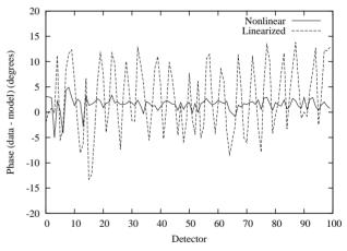
Figure 6: Difference in horizontal betatron phase advance between data and model with large closed orbit distortion after using a phase correction algorithm based on the linear (dashed) and nonlinear (solid) BPM evaluation.
