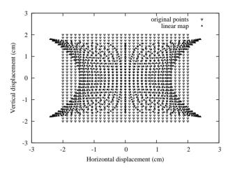
Figure 1: Distortion in CESR arc BPMs with approximately elliptical cross-section when linearization is used.
