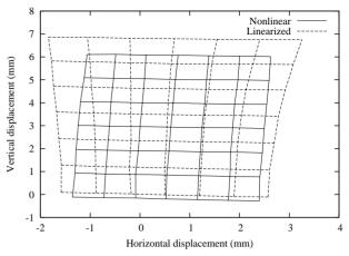
Figure 5: Separator scan. Orbits at detector 9W calculated using linearized (dashed) and nonlinear (solid) methods.
