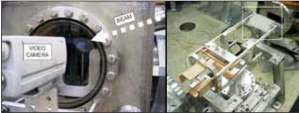
Figure 3: Pictures of the phosphor screen in the injection section (left) and in the extraction section (right).
