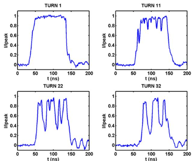
Figure 6: Longitudinal beam profiles measured with the Fast Faraday Cup when the beam is extracted after a variable number of turns.
