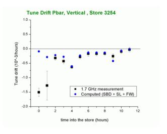
Figure 3: The antiproton tune drift during the store compared to expectation based on transverse and longitudinal emittance and intensity measurements
