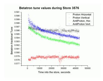
Figure 2: Proton and Antiproton fractional betatron tune during the store.
