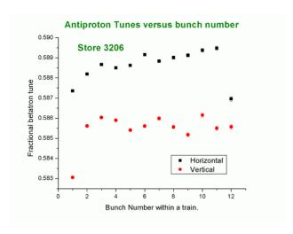
Figure 4: The antiproton tunes for all 12 bunches in the train, averaged over the three trains. The data was taken when tunes were fairly stable, staying only for a few minutes in a given gating configuration. The shift observed for the first and last bunches are signficantly larger than our statistic or systematic accuracy.
