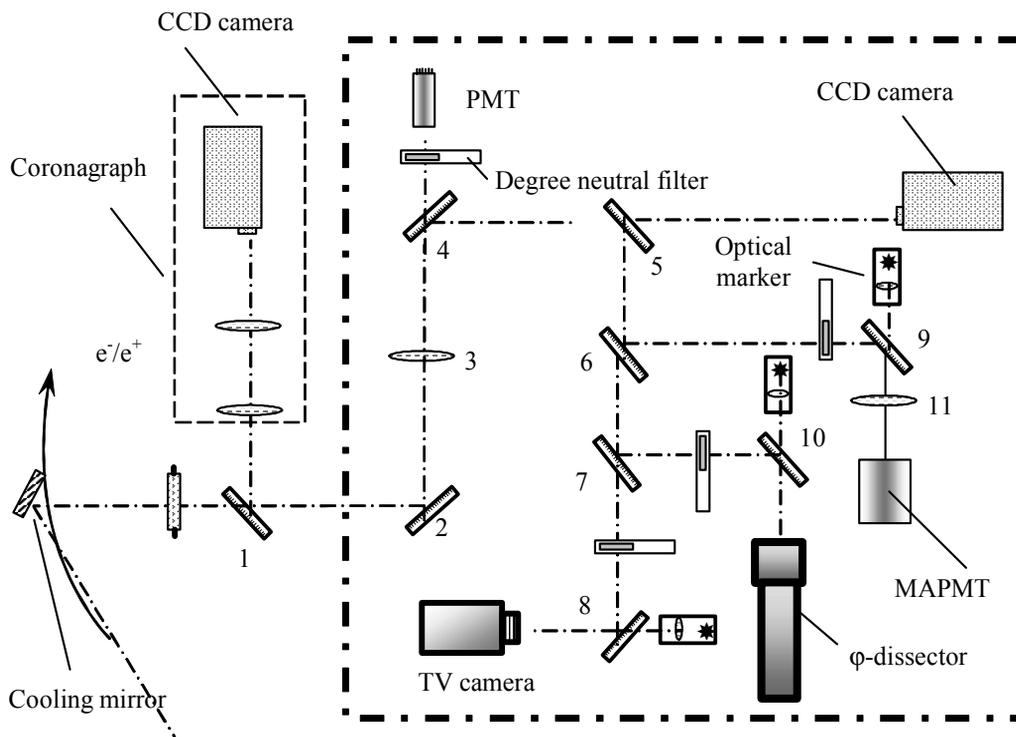
Figure 1: Layout of the optical diagnostic. 3,11 – lenses, 4+10 – mirrors
