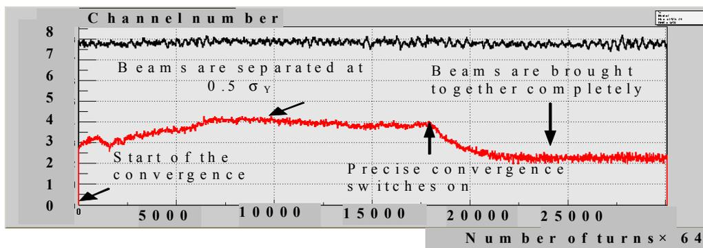
Figure 5: The position of center-of-weight of electron beam (upper line) and size  $\sigma_Y$  behavior (down line) during the beams convergence in the interaction point. The total process duration is nearly  $2 \cdot 10^6$  turns of the beams. Time of the single turn is 1220 ns. Channel constant is 0.12 mm.
