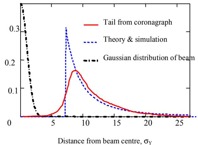
Figure 3: Measured and simulated beam tails distribution. Gauss distribution is given for comparison.
