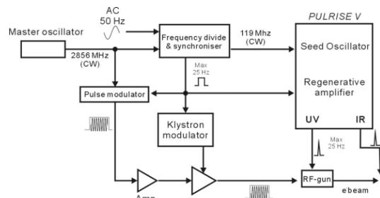
Figure 4: Block diagram of the synchronization system
