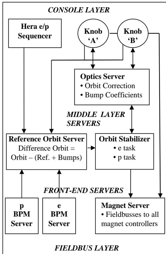
Figure 1: Communications for the orbit stabilization.
