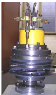
Figure 3: The modified duoplasmatron ion source and its lens system.
