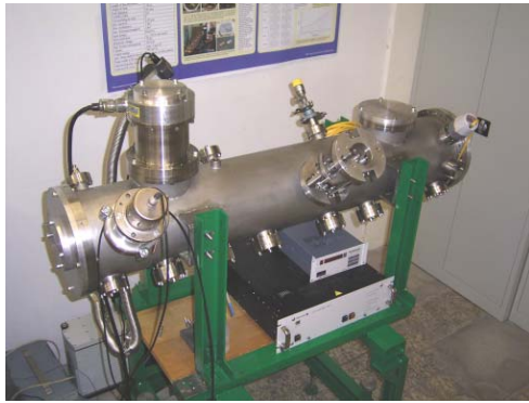
Figure 2: The RFQ-Tank ready for vacuum.
