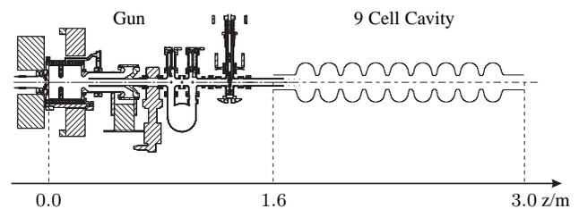
Figure 1: Layout of the examined structure consisting of a gun part and a subsequent TESLA 9-cell-cavity.
