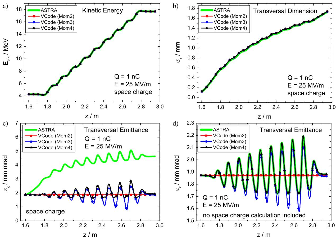
Figure 2: Simulation results for the cavity part of the examined test structure: a)-c) space charge forces are included; d) space charge forces are omitted.
