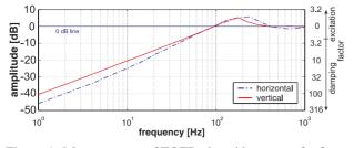
Figure 1: Measurement of FOFB closed loop transfer functions in both transverse planes. Effective damping of orbit perturbations has been achieved close to the FOFB design goal of 100 Hz.
