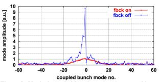
Figure 8: Vertical coupled bunch mode spectrum with active feedback system.
