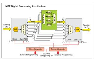
Figure 2: Digital filter structure
