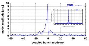
Figure 6: Central part of coupled bunch mode spectrum in the vertical plane using the multi bunch feedback as a passive diagnostic device (feedback loop not closed). In the insert, the total spectrum is shown.
