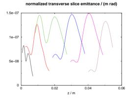
Figure 6: Transverse normalized slice emittance at different longitudinal bunch positions.
