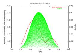
Figure 1: Slice emittance calculation from MAFIA data: Each green dot represents a single macro-particle. The red curve is the calculated slice emittance (slice width  $\sigma_z = 0.3$  mm). The projected normalized transverse emittance of the entire bunch is  $6.2496 \cdot 10^{-7}$  m·rad which is well above the values for the slice emittances.
